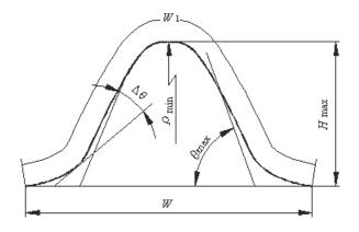
Figure 8. The evaluation method of wrinkle morphology.
