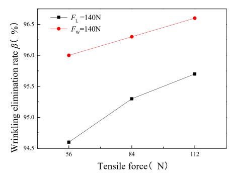
Figure 12. The relationships between the wrinkling elimination rate and tensile state of wrinkle.
