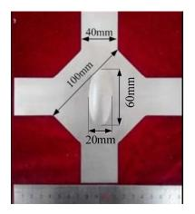
Figure 1. Wrinkling specimen.
