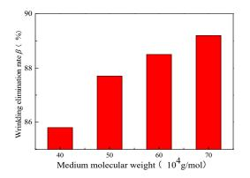
Figure 10. Relationship between the molecular weight of viscous medium and the wrinkling elimination rate.
