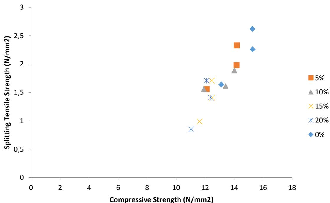
Figure 2. Relationship between the compressive strength and splitting tensile strength at all replacement levels.
