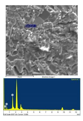
Figure 6. EDS spectrum of elements in the sample 2, magnification 2000x
