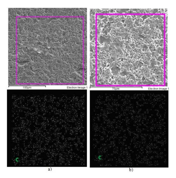
Figure 4. a) Distribution of carbon in the sample tested at magnification 500xb) Distribution of carbon in the sample tested at magnification 1000x
