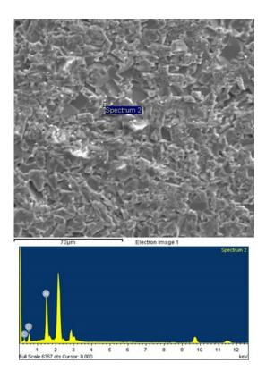
Figure 5. EDS spectrum of elements in the sample 2, magnification 1000x
