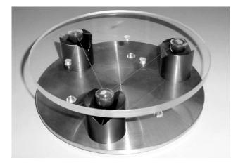
Figure 1. Maxwell kinematic mount.
