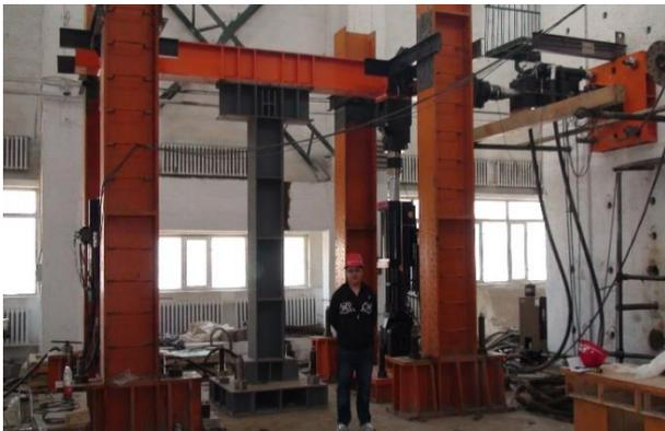
Figure 3. Test setup of 3 DOF testing system in HIT.
