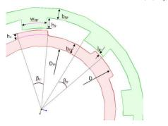
Figure 2. Parameters for SRM design
