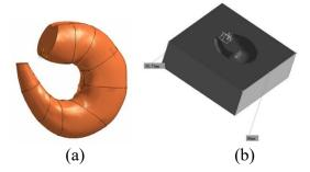
Figure 6. (a)The finished 3D model of shelled shrimp; (b)The finished cavity plate of shelled shrimp.
