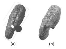
*Figure 4. (a) The point clouds are to be filled holes. (b) Filled holes in point clouds.*
