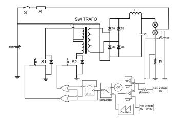
Figure 5. Push-Pull DC/DC power converter with current and temperature regulation.
