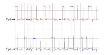
Figure 7. LED driver waveforms during LED light temperature change with current and temperature regulation (control signals of transistors S<sub>1</sub>, S<sub>2</sub>, 10 V/div., 50µs/div).
