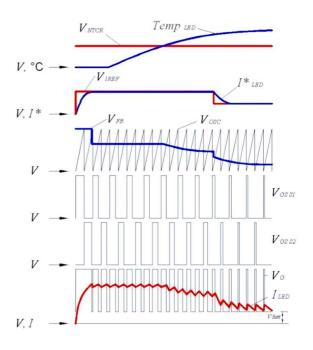
Figure 6. Principal LED driver waveforms for a step LED light temperature increase.
