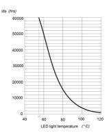
Figure 4. Durability of LED lighting versus operating temperature [21].
