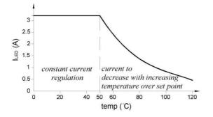
Figure 8. LED current versus its temperature.
