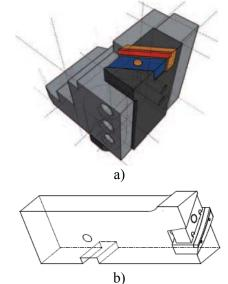
Figure 4. The rotational turning tool mountable into a turret of a lathe: a) 3D view of the tool, b) design of the tool [15].
