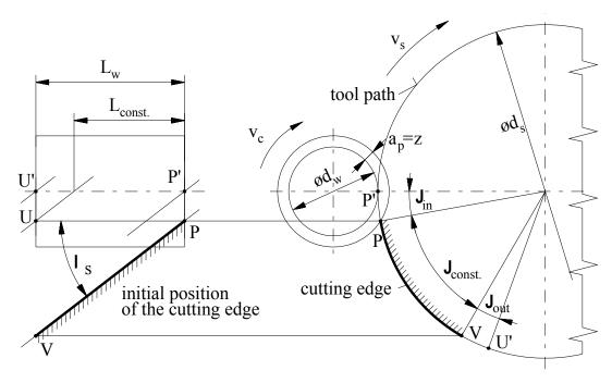
Figure 3. The four specific positions of the cutting edge and the needed rotation angles.
