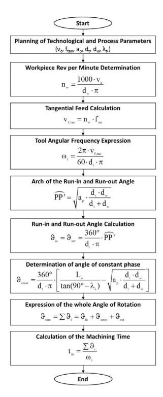
*Figure 6. Algorithm of the machining time calculation.*
