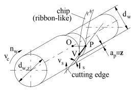
Figure 2. The principle of material removal in rotational feed turning.
