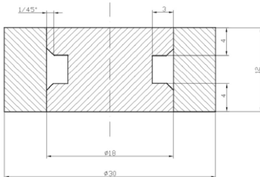
Figure 5. Dimensions of bimetallic components
