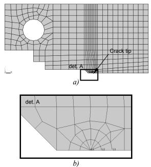
Figure 5. a) FE model of CT specimen. B) Detail of FE mesh around crack tip
