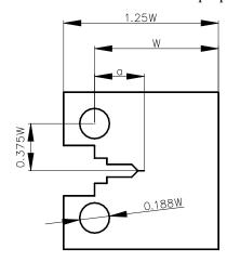
Figure 4. Geometry and dimension of CT specimen
