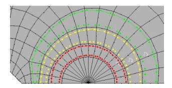
Figure 2. *J*-integral contour paths  $(\Gamma_1, \Gamma_2, \Gamma_3)$  surrounding the crack tip through the integration points of finite elements
