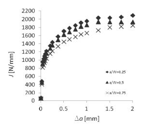
Figure 7. AISI 420: predicted J values for crack extension Δa
