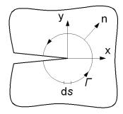
Figure 1. J-integral arbitrary contour path enclosing the crack tip
