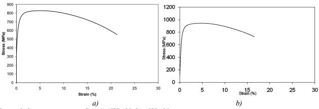
Figure 3. Stress-strain curve for: a) AISI 420. b) AISI 431.
