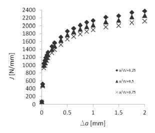
Figure 8. AISI 431: predicted J values for crack extension Δa.
