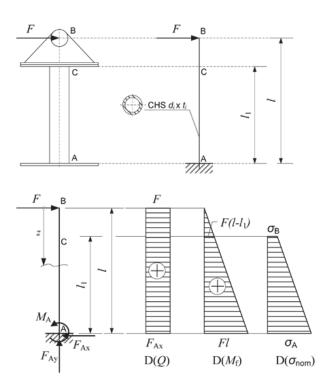
Figure 2. Analytical model with diagrams for stress, bending moment and transversal force
