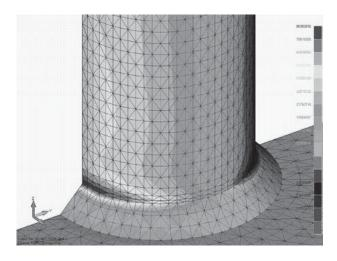
Figure 10. FEM stress concentration of normal stress in z-direction
