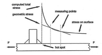
Figure 3. Structural stress definition [3, 7]
