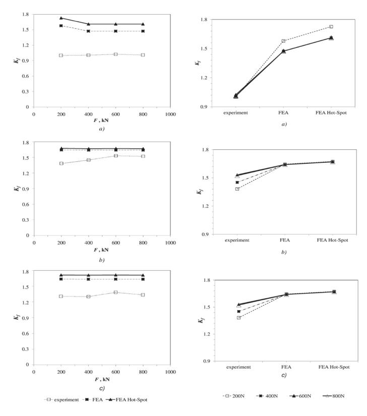
Figure 13. Dependency of stress concentration factor values in respect to loading level
