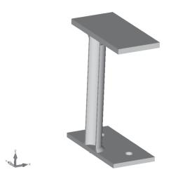
Figure 7. Half model of CHS-plate T-joint
