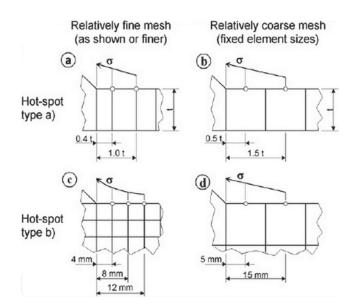
Figure 6. Reference points for different types of meshing [3]
