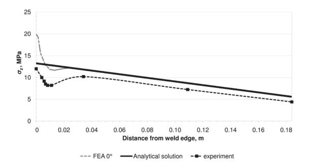
Figure 12. Stress distribution in bending plane
