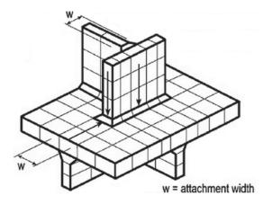
Figure 5. Typical mesh and stress evaluation paths for a welded detail [3]
