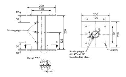
Figure 1. Geometry of CHS-plate T-joint with strain gauge positions for acquiring experimental data [6]
