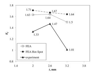
Figure 15. Comparison of stress concentration factors for different wall thicknesses
