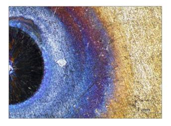
Figure 2. Heat tints after dotted TIG heat input on samples prepared for testing according to ASTM 61.
