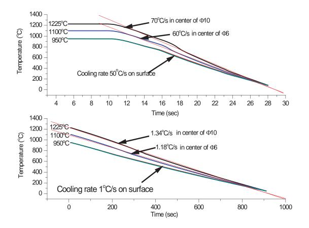
Figure 3. Temperature and cooling rate in the specimen
