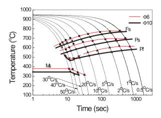
Figure 1. CCT curves of the Ø6 mm and Ø10 mm specimens, where Fs - ferrite start; Ps pearlite start; Pf - pearlite finish; Ms martensite start
