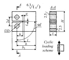
Figure 1. Compact specimen for testing under cyclic normal tension
