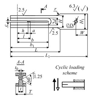
Figure 2. I-beam specimen for testing under cyclic transverse shear
