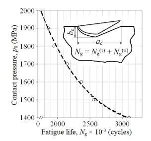
Figure 5. Residual life curve of  $65\Gamma$  steel based on the criterion of the spall formation
