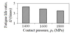
*Figure 6. Fatigue life ratios of compared steels at different contact pressures*
