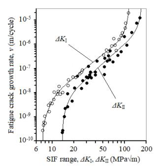
Figure 4. Fatigue crack growth rate curves of  $65\Gamma$ steel ( $\sigma_{0.2} = 830$  MPa) built considering crack faces friction
