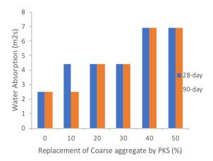
Figure 13. Sorptivity and water absorption of lateritic concrete with PKS
