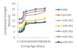
Figure 4. Compressive strength development of lateritic concrete with PKS
