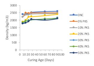
Figure 3. Density characteristics of lateritic concrete with PKS
