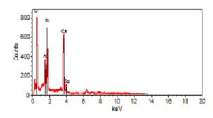
Figure 12. EDX spectrum of lateritic concrete with 20% PKS
