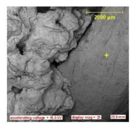
Figure 6. SEM micrograph of lateritic concrete with 10% PKS
