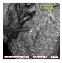
Figure 7. SEM micrograph of lateritic concrete with 20% PKS
