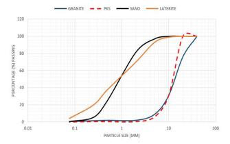
Figure 2. Particle size distribution of the aggregate, PKS and laterite
