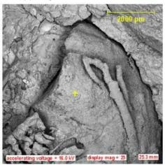
Figure 8. SEM micrograph of lateritic concrete with 40% PKS
