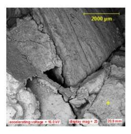
Figure 9. SEM micrograph of lateritic concrete with 50% PKS
