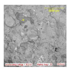
Figure 5. SEM micrograph of lateritic concrete with 0% PKS
