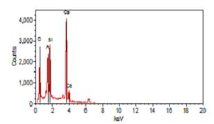
Figure 11. EDX spectrum of lateritic concrete with 10% PKS
