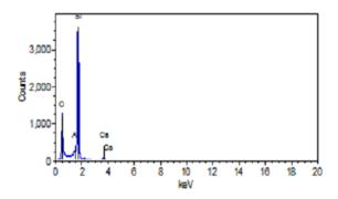
Figure 10. EDX spectrum of lateritic concrete with 0% PKS
