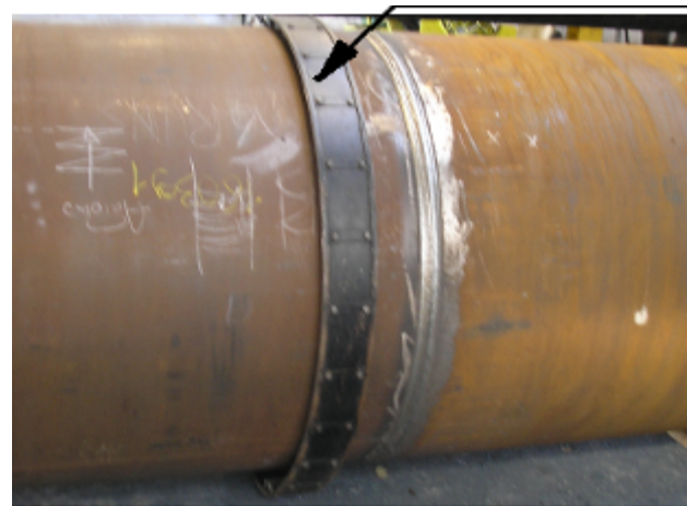
Slika 2. Montirani prsten – zupčasta letva Figure 2. Circular rigid rail mounted on a pipe
