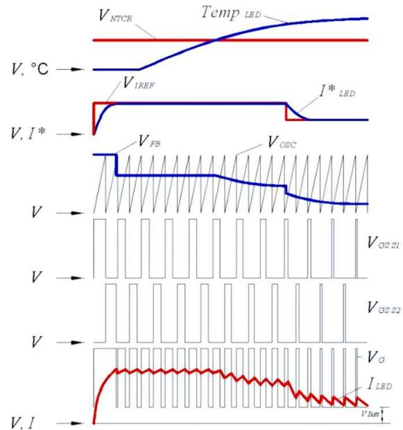
Figure 6. Principal LED driver waveforms for a step LED light temperature increase.
