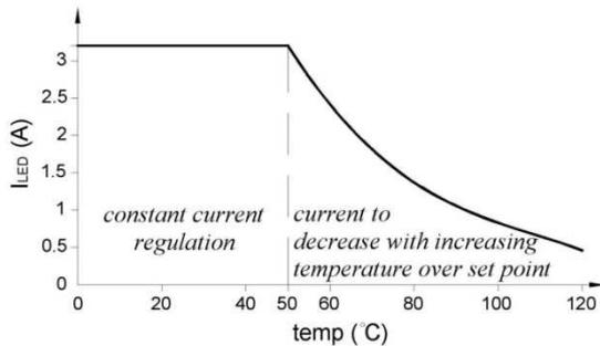
Figure 8. LED current versus its temperature.
