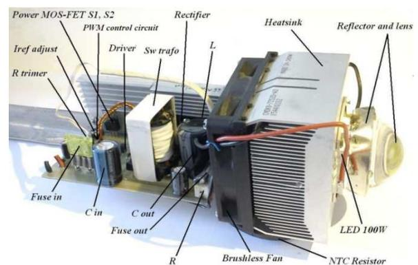
Figure 9. 100W hand light with DC/DC converter.
