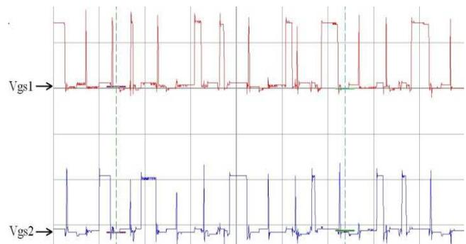
Figure 7. LED driver waveforms during LED light temperature change with current and temperature regulation (control signals of transistors  $S_1$ ,  $S_2$ , 10 V/div., 50 $\mu$ s/div).
