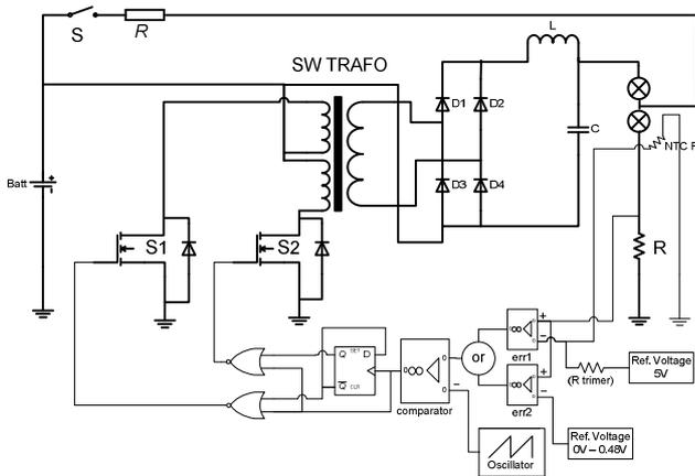
Figure 5. Push-Pull DC/DC power converter with current and temperature regulation.
