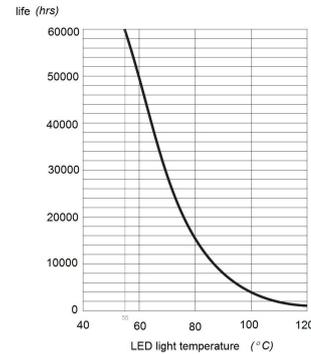
Figure 4. Durability of LED lighting versus operating temperature [21].
