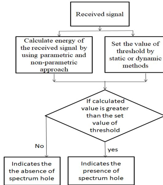
Figure 5. Flow chart for energy detector spectrum sensing technique.
