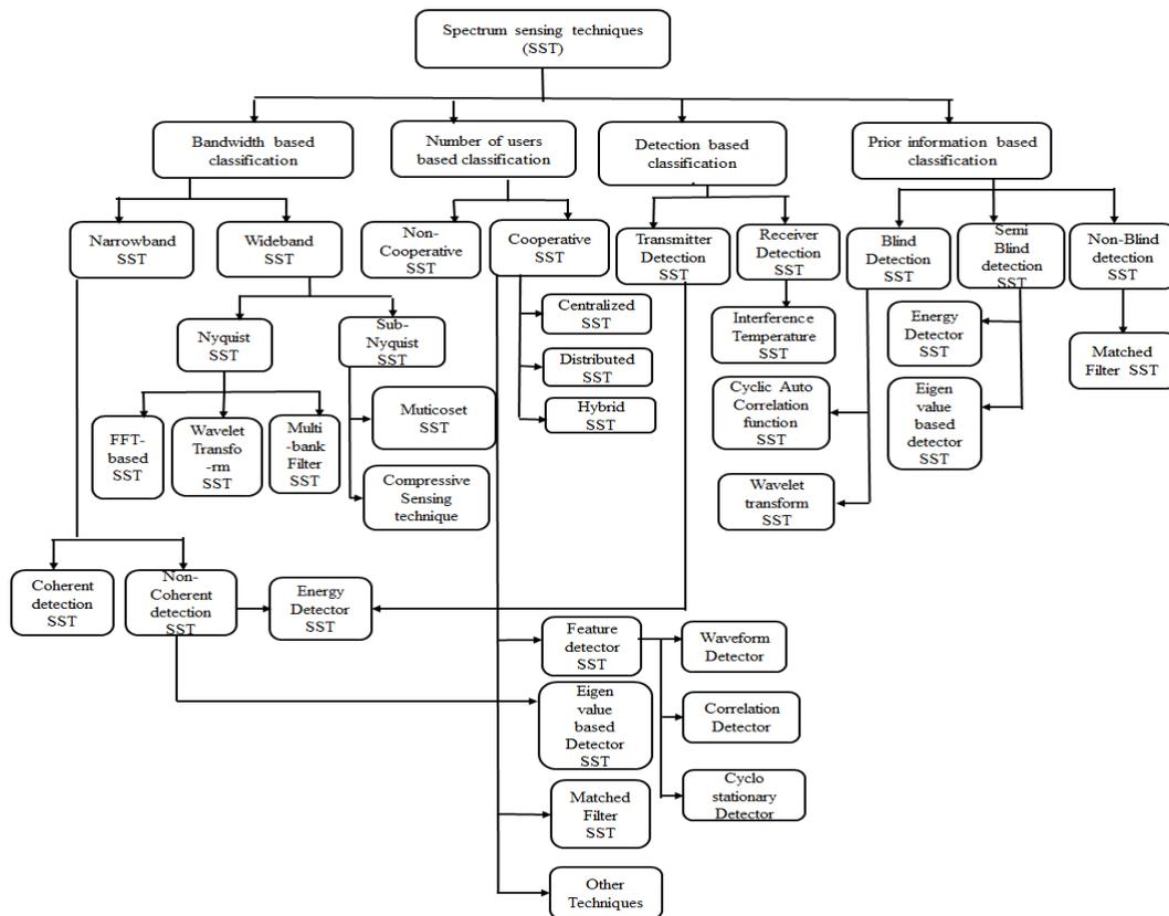
Figure 3. Classification of spectrum sensing techniques.
