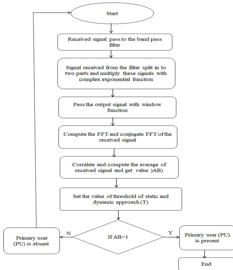
Figure 9. Flow chart for cyclostationary feature detector spectrum sensing technique.
