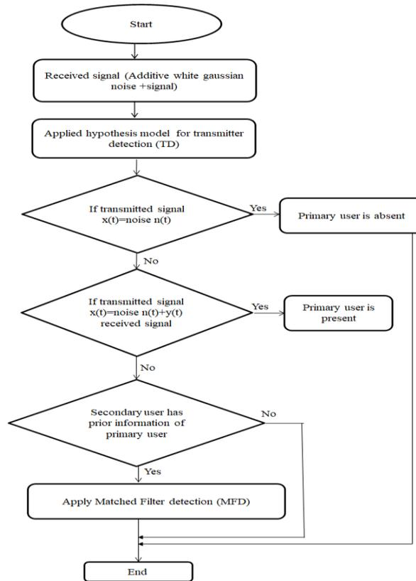
Figure 7. Flow chart for matched filter detector spectrum sensing technique.
