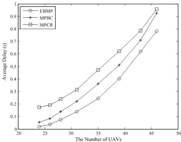
Figure 9. Average delay versus the number of UAVs.
