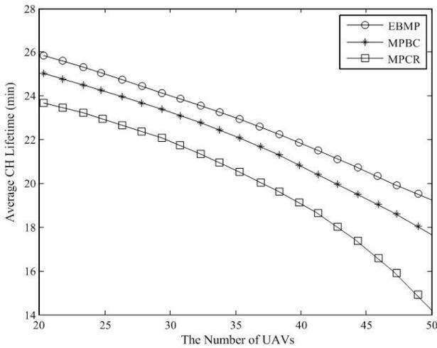
Figure 6. The average CH lifetime versus the number of UAVs.
