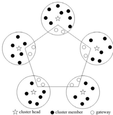
Figure 1. The hierarchical network of the cluster structure.
