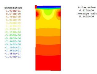
Figure 5. The temperature field of XY section of refrigerated warehouse floor while air velocity is 3.5m/s.
