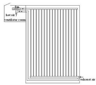
Figure 1. The schematic diagram of the overall ventilation system.
