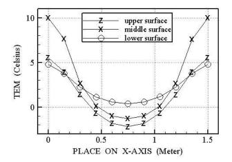
Figure 9. The temperature curves of points on upper, middle, and lower surface for heating layer while air velocity is 1.5m/s.
