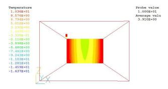
Figure 7. The temperature field of middle surface for heating layer while air velocity is 3.5m/s.
