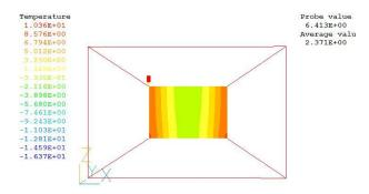
*Figure 6. The temperature field of upper surface for heating layer while air velocity is 3.5m/s.*
