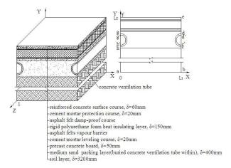
*Figure 2. The calculating element of heat-transfer model for refrigerated warehouse floor.*
