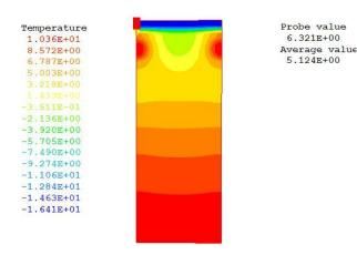
Figure 4. The temperature field of XY section of refrigerated warehouse floor while air velocity is 2.5m/s.
