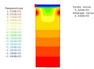
Figure 3. The temperature field of XY section of refrigerated warehouse floor while air velocity is 1.5m/s.
