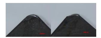
Figure 8. Wear of insert IN23 f = 0.2mm (left), f = 0.32 mm; 1 plate [1].
