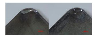
Figure 13. Wear of insert D460 f = 0.2 mm (left), f = 0.32 mm; 4 slates [1].
