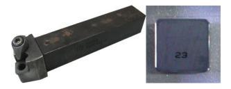
Figure 3. Tool holder CSRNR 25 x 25 and insert ISCAR IN23 [1].
