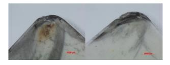
Figure 11. Wear of insert D210 f = 0.2 mm (left), f = 0.32 mm; 1 slat [1].
