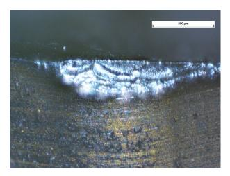
Figure 4. Surface morphology of worn cutting insert investigated with optical microscope Nikon Eclipse LV100ND (50x).
