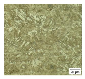
Figure 1. Microstructure of Hardox 500 in "as delivered" state.
