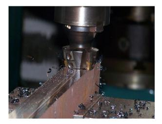
Figure 2. An overall view to rough face hard milling process of Hardox 500 steel.
