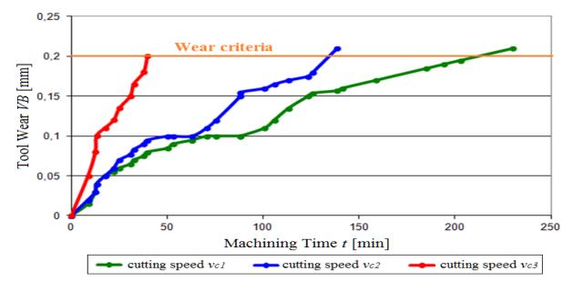
Figure 5. Graphical presentation of dependence of tool wear on machining time in rough milling of Hardox 500 steel with cemented carbide cutting tool inserts to determine the dependence of  $T = f(v_c)$ .
