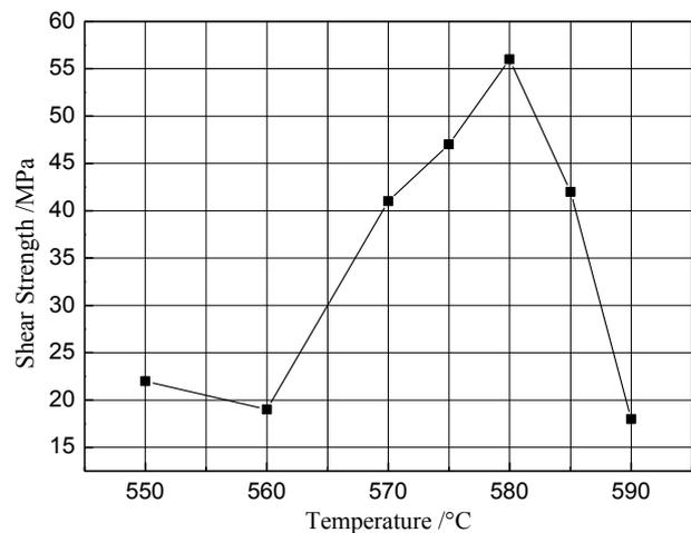
Figure 5. Shear strength of the joint brazed at different temperatures with soaking time 30 min.
