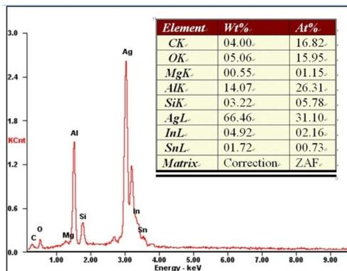
Figure 4. Point scanning analysis of white area in SiC<sub>p</sub>/6063Al MMCs with soaking time 30 min at 580 °C,
