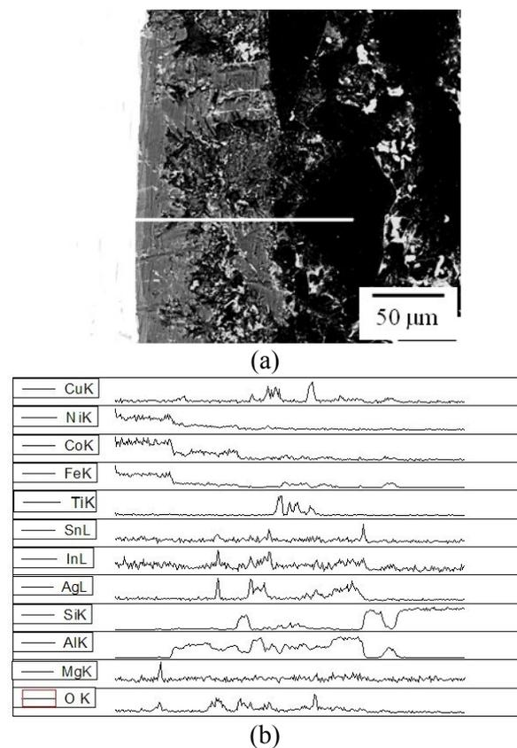
Figure 3. Line scanning analysis of brazing seam with soaking time 30 min at 580 °C: (a) location and (b) results.
