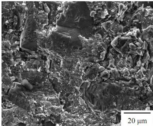
Figure 6. Fracture morphology on the side of  $\text{SiC}_p/6063\text{Al}$  MMCs.
