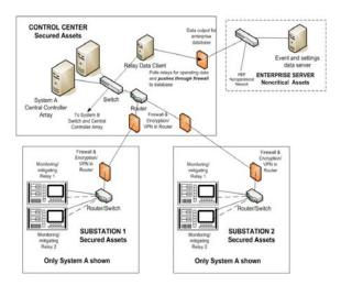
Figure 10. Secure communications architecture
