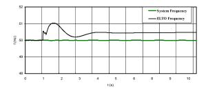
Figure 9. System and sub-system frequency response, an islanding scenario with generation surplus
