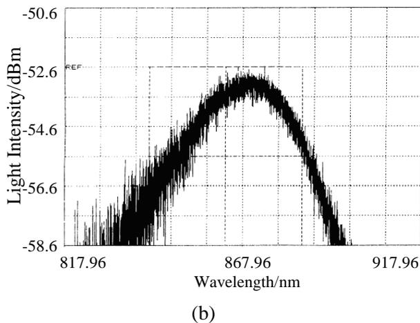
Figure 3. Luminescent spectrums under different temperature stress: (a) Device 04 light source 1 (100), (b) Device 31 light source 1 (175).
