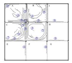
Figure 9. Crack pattern on the top of panels.
