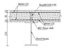
Figure 2. Cross-section of composite beam.
