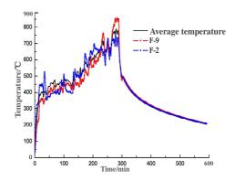
Figure 5. Recorded furnace gas temperatures.
