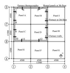
Figure 1. Location of test panels under fire.
