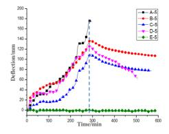
*Figure 8. Vertical deflection at central part of each panel.*
