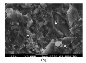
Figure 5. Fracture appearance on both sides of the composite (a) under low magnification view; (b) under high magnification view.
