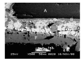
*Figure 4. The microstructure of the soldered joint in the soldered seam.*
