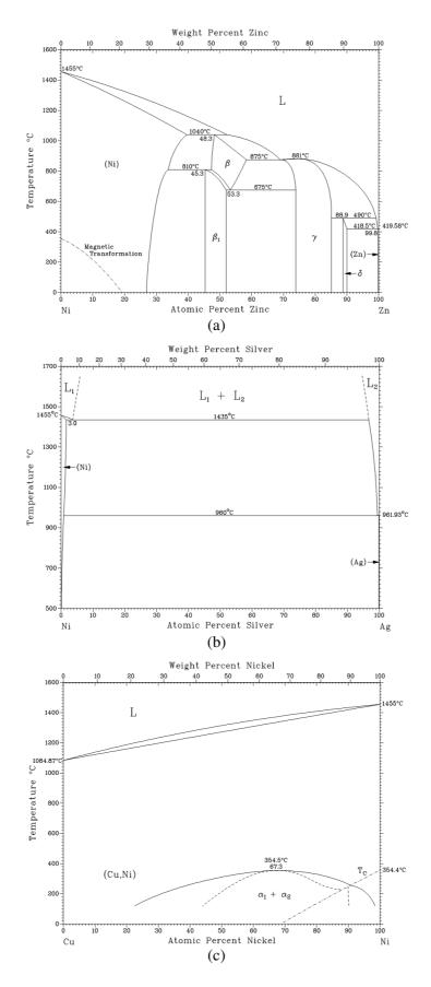
Figure 2. Binary alloy phase diagram (a) Zn-Ni (b) Ag-Ni (c) Cu-Ni.
