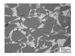
Figure 1. The original structure of Al-MMCs.
