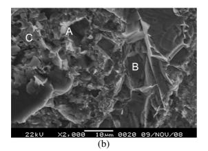
Figure 6. Fracture appearance on the side of filler metal (a) under low magnification view; (b) under high magnification view.
