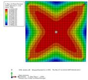
Figure 3. The maximum principal stress of the new panel.
