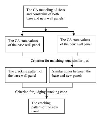
Figure 2. The procedure for the CA method.
