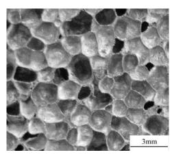
Figure 1. A macroscopic view of the closed-cell Al foam, used in the current study.
