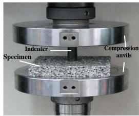
Figure 2. Indentation test setup of Al foam.
