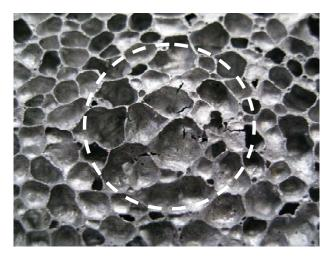
Figure 6. Macrographs of Al foam back region for simple boundary condition under the FEP indentation with depth of 6mm.
