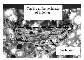
Figure 7. Cross-sectional morphology of Al foam after indentation.
