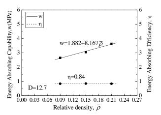
Figure 12. w-  $\overline{\rho}$  and  $\eta$  -  $\overline{\rho}$  curves of Al foam.
