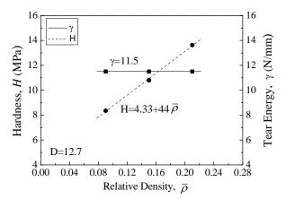
Figure 11.  $H - \overline{\rho}$  and  $\gamma - \overline{\rho}$  curves of Al foam.
