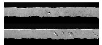
Figure 9. Longitudinal sections of the butt-welded specimens obtained with focused beam (up) and defocusing to -1 mm (down)
