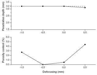
Figure 8. Penetration depth and porosity content as function of focus position
