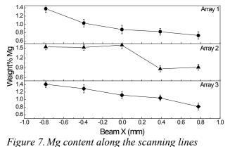
From the results obtained in site 2 and 3, it is possible to point out that Mg concentration decreases moving from the base material towards the melted zone.
