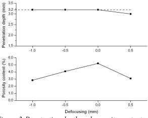
Figure 3. Penetration depth and porosity content as function of focus position
