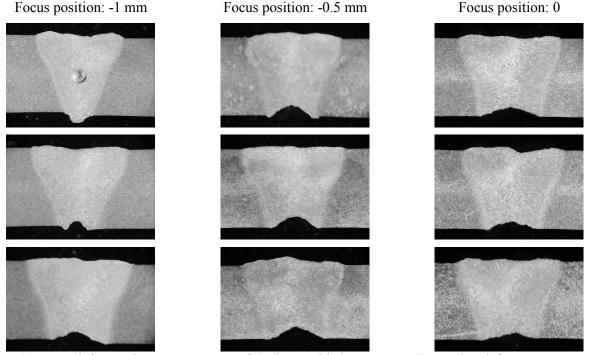
*Figure 10. From left to right, cross sections of the butt welded specimens obtained with focus position to -1, -0.5 and 0 respectively; sections listed from up to down following the welding direction*
