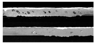
Figure 4. Longitudinal sections of the specimens obtained with focused beam (up) and defocusing to -1 mm (down)
