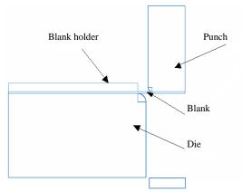
Figure 3. The geometric model of the U-shaped parts achieved by hot contact bending.
