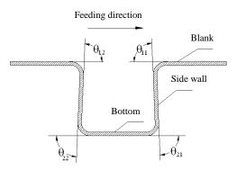
Figure 2. The definition of various parts at the hot stamping pieces.
