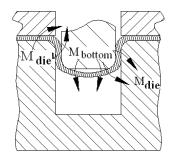
a) Springback caused by the forming force
