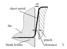
Figure 7. Diagram of the wedge angle  $\alpha$ .
