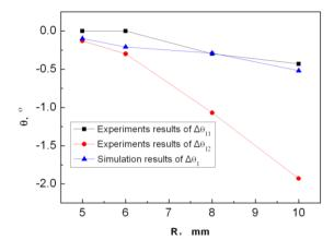
Figure 6. The relationship between the die radius and springback  $\Delta \theta_1$ .
