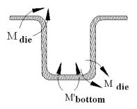
b) Springback caused by hot contact bending
