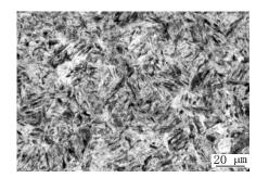
Figure 5. Microstructure of ultra-high-strength boron steel stamping parts.
