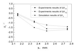
*Figure 8. The relationship between the die clearance and springback.*
