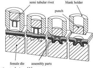
Figure 1. Self-piercing riveting technique [1]
