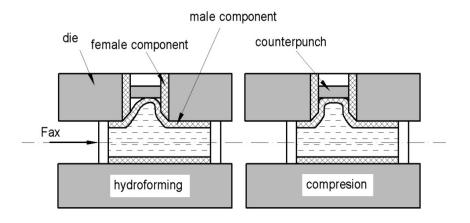
Figure 2. Angular joining by hydroforming [2]
