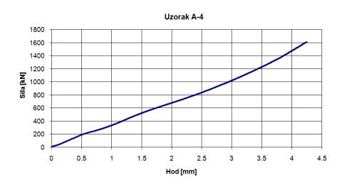
Figure 9. Load – stroke characteristic for the model A-4
