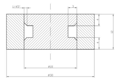
Figure 5. Dimensions of bimetallic components
