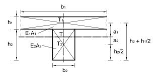
Figure 4. Eccentricities of the layer's axis of centroids with respect to the axis of centroids of the fully composite beam.
