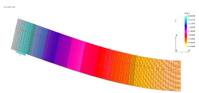
Figure 6. A finite element model for the composite timber-EPS specimen.
