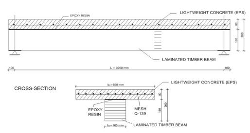
*Figure 1. Tested composite timber-concrete beam specimen [2].*
