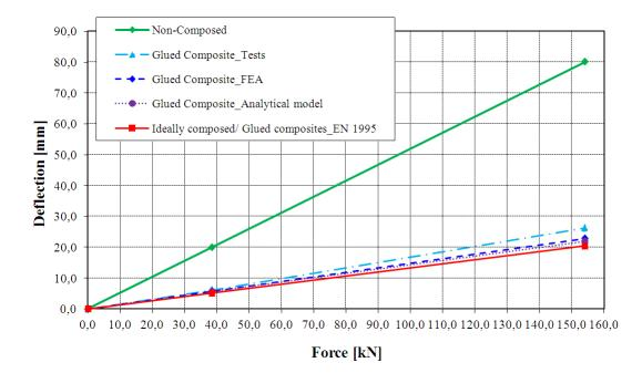
Figure 8. A comparison of the results obtained by different analyses (force-deflection diagram).
