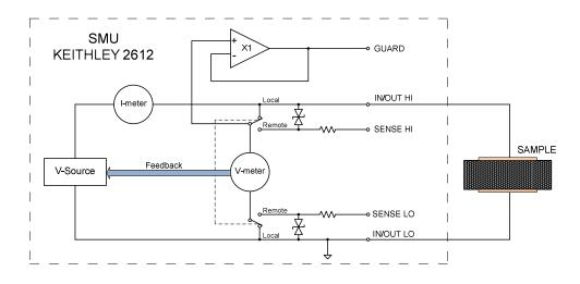
*Figure 3. Measurement of insulation resistance at constant voltage*
