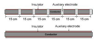
Figure 4. Lateral section of the Corkscrew electrode with measuring points marked (up); Lateral section of the electrode with auxiliary electrode (down).
