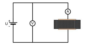
Figure 2. Classic U-I method for measuring volume resistance of the sample
