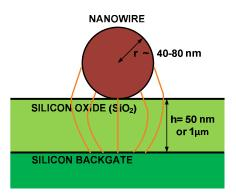
Figure 5. Schematics of the GaAs nanotransistor cross section. Orange lines represent electrical field in back-gate capacitor. Geometrical relations are exaggerated for the sake of clarity
