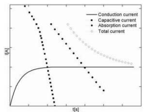
Figure 1. Total current density versus the time for the dielectric material[3]
