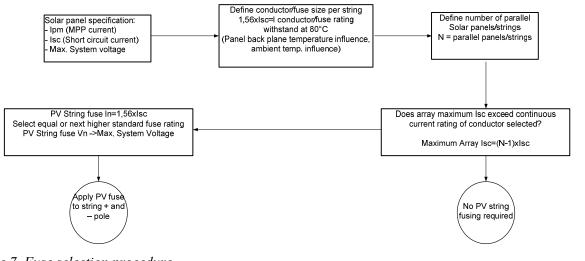
Figure 7. Fuse selection procedure
