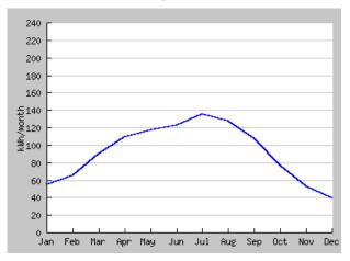
Figure 3. Estimation of PV system electric energy monthly production – PVGIS, [4]
