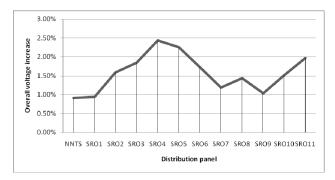
Figure 14. PV generator operation impact on LVDN voltage increase – open loop form operation
