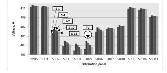
Figure 10. Voltage profiles at maximum LVDN loading
