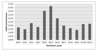
Figure 18. Fault current relative increase due to PV system operation – open loop form
