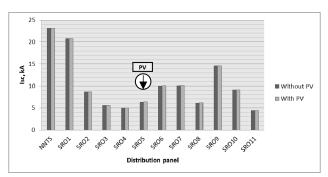
Figure 17. LVDN triphase fault currents – open loop form operation
