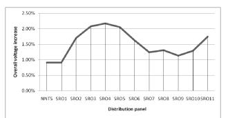
Figure 13. PV generator operation impact on LVDN voltage increase – closed loop form operation
