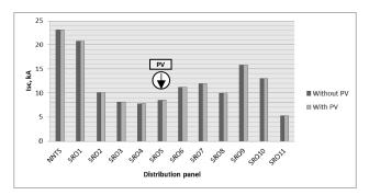
Figure 15. LVDN triphase fault currents – closed loop form operation
