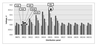
Figure 12. Voltage profiles at LVDN no-load conditions
