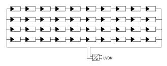
Figure 5. PV system with central inverter, U>120Vdc
