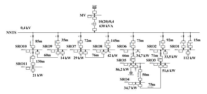
*Figure 9. Power factory model of a real low voltage distribution network – PV system connected at node SRO5*
