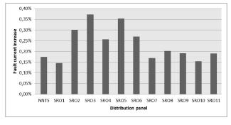
Figure 16. Fault current relative increase due to PV system operation – closed loop form
