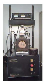
Figure 5. Marshall stability and flow test equipment
