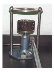
Figure 4. Marshall Specimen Extractor
