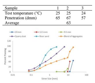
Figure 3. Particle size distribution curves of the aggregates and blend of aggregates for the asphalt concrete
