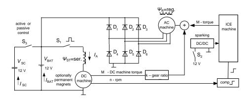
Figure 4. Simplified schematic of conventional car which enables simulation of different energy storage systems during cranking.
