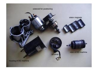
Figure 7. DC machine after disassembly; after the numerous cranking tests stator field magnets were displaced and rotor was damaged, brushes were practically vanished as a consequence of extensive use.
