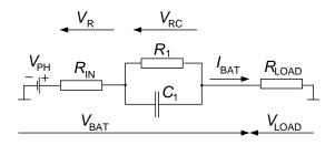
Figure 2. Simplified schematic of Lead-acid battery connected to the load.
