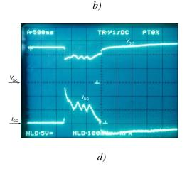
Figure 6. Measured waveforms of DC bus voltage and current of the energy storage system during cranking; a) lead-acid battery cranking, b)lead-acid battery with Li-ion battery and electrolytic capacitor cranking, c) supercapacitors unsuccessful cranking, d) successful cranking with supercapacitors (100 A/div., 5 V/div., 500 ms/div.).
