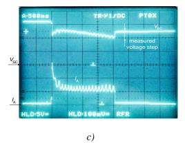
simulated that battery enables successful cranking for 12 V (Figure 5.a and Figure 6.a) but supercapacitors not because of rapid discharging and increased voltage drop during cranking (Figure 5.b and Figure 6.c).
