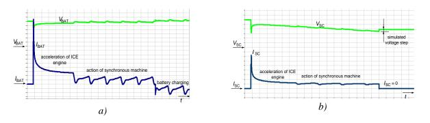
Figure 5. Simulated waveforms of DC bus voltage and current of the energy storage system during cranking; a) lead-acid battery successful cranking, b) supercapacitor unsuccessful cranking (25 A/div., 2 V/div., 100 ms/div.).
