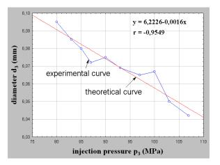
Figure 4. Influence of the injection pressure  $p_3$  change on diameter  $d_3$  of the product
