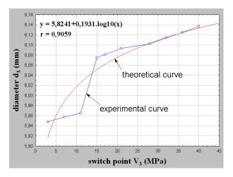
Figure 7. Influence of the switch point  $V_3$  change on diameter  $d_3$  of the product
