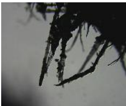
Figure 1. An example of mechanical degradation of paper insulator - enlarged by optic microscope by the factor of 10 (Laboratory for Marine Electrical Engineering, Faculty of Maritime Studies in Split).
