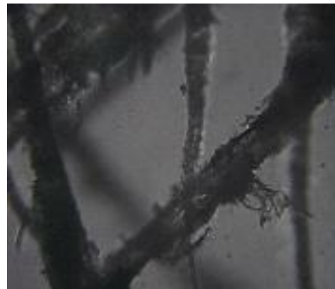
Figure 2. Paper - enlarged by microscope by the factor of 40 (Laboratory for Marine Electrical Engineering, Faculty of Maritime Studies in Split).
