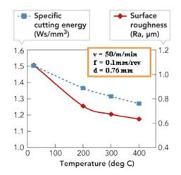
Figure 5. The Effect of temperature exerted on Specific cutting energy and surface roughness [58].
