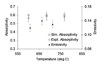
Figure 2. The effect of temperature on absorptivity and emissivity [58].
