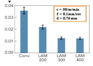
*Figure 4. Tool wear vs. temperature [58].*
