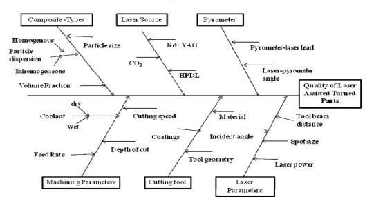
*Figure 6. Ishikawa cause-effect diagram of a laser assisted turning process.*
