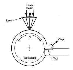
Figure 1. A schematic representation of laser assisted machining [59].
