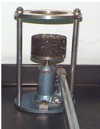
Figure 4. Marshall Specimen Extractor
