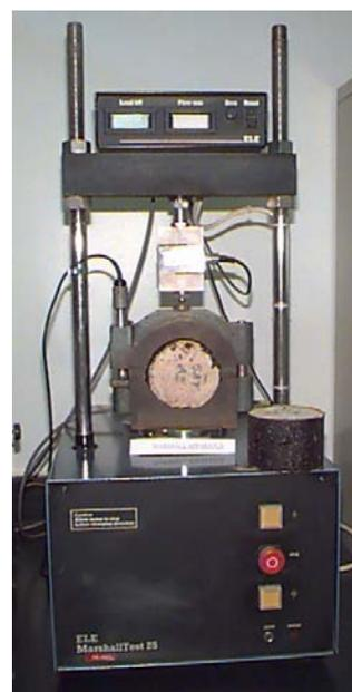
Figure 5. Marshall stability and flow test equipment
